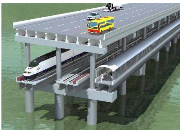
Conceptual Drawing/ I-244 Multimodal Bridge (to accommodate Study Recommendations), drawing by Garver Engineering/ODOT State of Oklahoma Passenger Rail Study, USA
